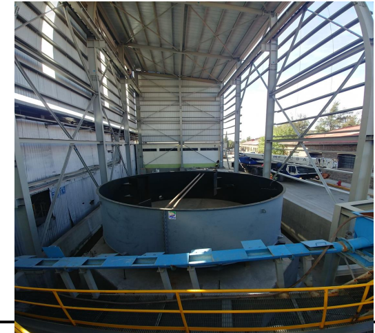
Zn Flotation cell (300 m 3 )
